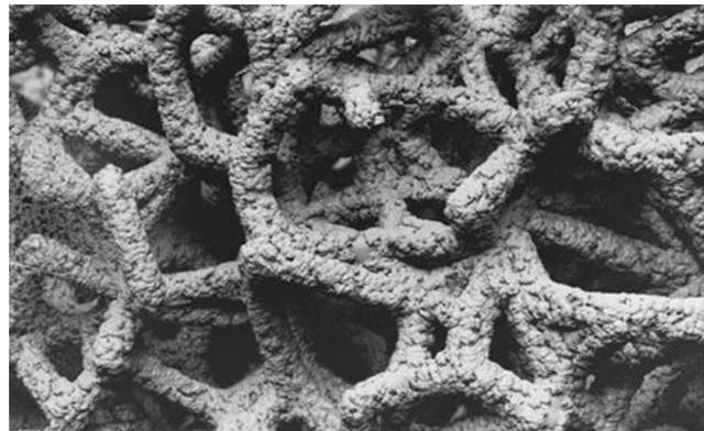
**Fig. 1.** Surface microstructure of a custom implant (magnification x40)
